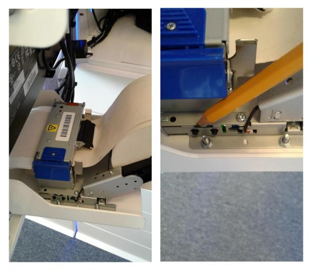
Close the arm until it attaches back to the printer (above). To feed the receipt paper through, press the small black button as indicated by the pencil in the picture above.
