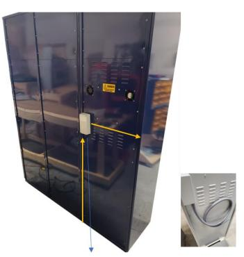
Cable to exit from under waterproof box The box is 41" from floor level and 19" from the side of the cabinet
