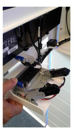
Press the **blue button** on the left of the printer to release the arm (above).
